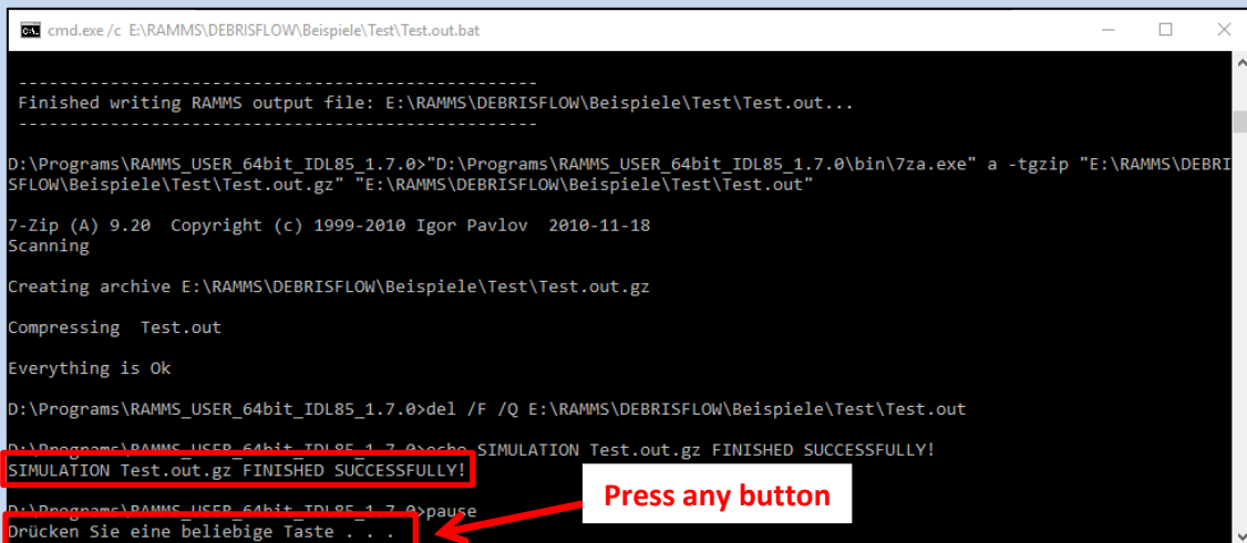
Figure 3. 3-58: Background simulation mode window. Press any button to close the DOS window.
