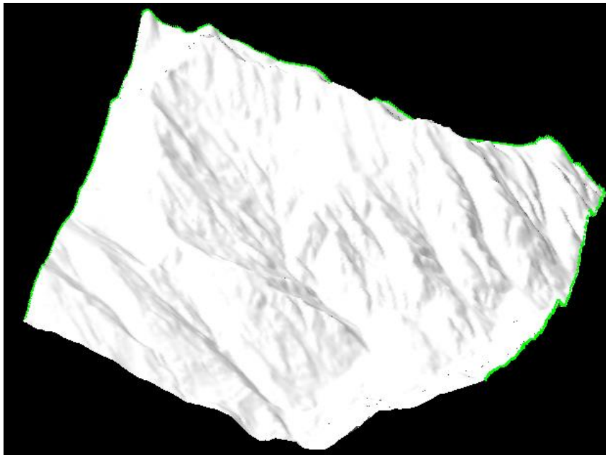
Figure 3-23 DEM surface visualization (with shadows) after creating a new project in RAMMS
