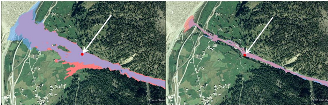
Figure 5-3: Comparison of the inundated areas of a simulation with a block release and a hydrograph (left) for a volume of 200'000 m 3 and (right) a volume of 2'250 m 3 . For all simulations \mu=0.225 and \xi=130 m/s 2 . Blue: hydrograph, red: block release. The red points indicate the location of the measured discharge curves (Figure 5-2).
