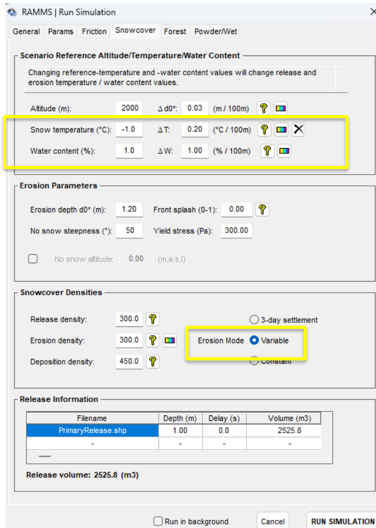
Figure 8.1: Example of the input specification of a wet snowcover. In this case 1% water is defined at an elevation of 2000m. The height of the snowcover at 2000m is 1.20m, thus there will be 12.00mm of water in the snowcover. Because snow height gradients are defined, the amount of water content will vary with elevation. Typically, with wet snow avalanche, higher densities are applied, in the case \rho_{\Sigma}=300\text{kg/m}^3 . We define the older snowcover using the Variable method. Also note that the splash parameter is set to 0.
