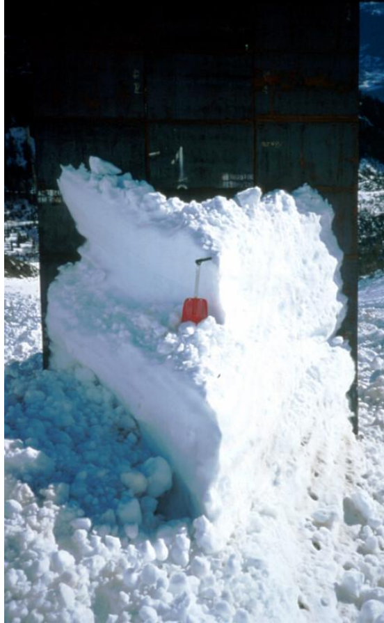
Figure 6.18: Example of wedge-shaped pile-up at the Vallée de la Sionne test site in 1998. A wet snow avalanche hit a 3.5m wide wall with an approximated velocity of 5m/s. The compacted snow densities in the wedge ranged from 500kg/m 3 to 550 kg/m 3 . The wall is 7m high. The wall was later destroyed by large avalanches that occurred several months later in January and February 1999. Note the symmetry of the wedge. The wedge angle appears to approximately \alpha_1 = 30^\circ ( 2\alpha_2=60^\circ ). Picture Gauer, SLF.
